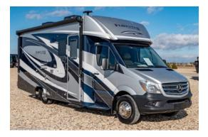
The <u>Class C (mini) Motorhome</u> provides many of the luxuries and conveniences of a Class A Motorhome in a scaled-down and less expensive unit. They are built on an automotive van chassis designed expressly for the Class C.
