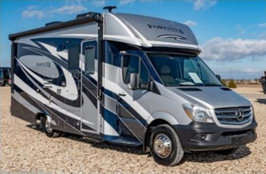
The **Class C (mini) Motorhome** provides many of the luxuries and conveniences of a Class A Motorhome in a scaled-down and less expensive unit. They are built on an automotive van chassis designed expressly for the Class C.
