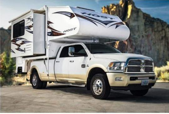
The **Truck Camper** is loaded onto the bed of a pickup truck and is very popular for remote location camping. Some newer units even have a slide-out for increased living space. Truck Campers are ideal units for those who already own a truck, making the transition to the world of RVing much easier.
